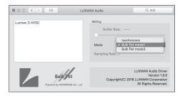
While music data is played back, the sound is interrupted or noise is generated owing to underperforming PC. In this case, the problem may be resolved by opening "LUXMAN Audio Driver Control Panel" in the "Control Panel" and increasing the buffer size with use of the slider.
