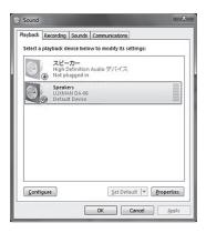
If you would like to output only playback sound of music files from the D/A converter connected to a PC using a music playback software\* applicable to Windows exclusive mode, select a device other than the connected model from the playback devices described above with "Set Default" button. In this case, the Windows event sound (alarm and incoming mail tone) selected in the "Sound" tab is not provided from the connected D/A converter or CD/SACD player with USB input.
